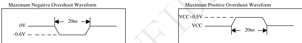
Figure 5-1 Maximum Overshoot Waveform
